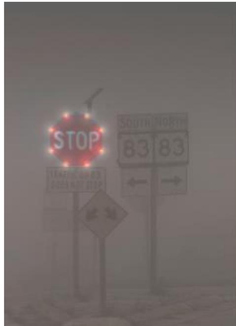
*Photo of LED Blinker Stop sign in fog courtesy of TAPCO.*
